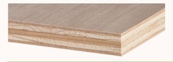
J Classic Core is constructed with a Classic Lam, pre-sanded platform before application of the face and back veneers and another trip through the press and sanding line, referred to as "two-step" construction. This platform fits the bill for end users that operate CNC equipment that requires tighter tolerances. For end users that need a core that is even closer to a full 3/4" Columbia offers a 19.5 mm (.767) J Classic Core construction option.
